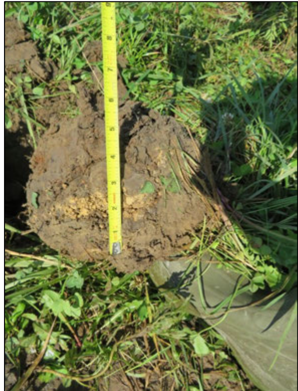
Sample Point 3-1, second soil sample: mixed, disturbed soils with gravel fill materials. Note light colored gravel lens.
